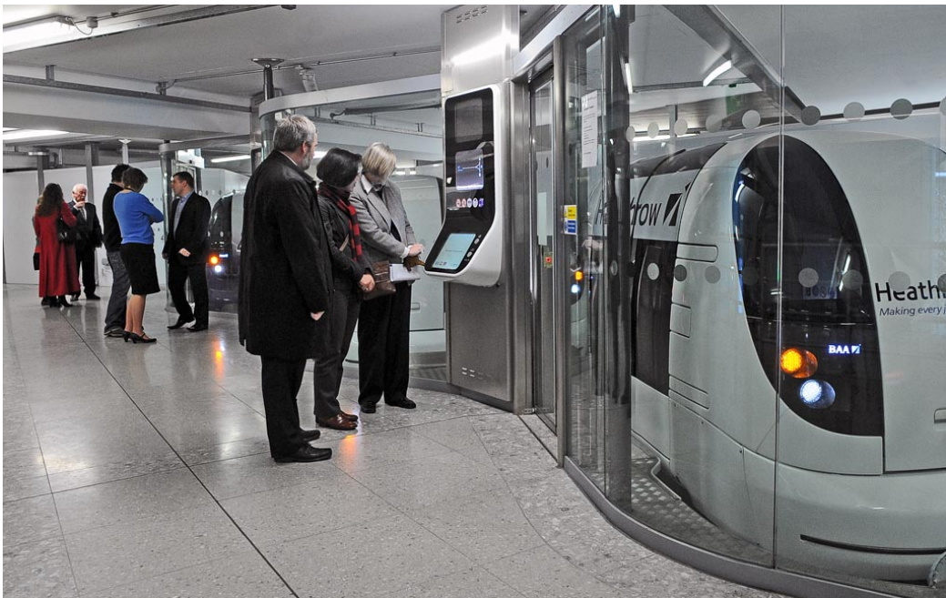
Figure 1.6: Passengers at berths in the Terminal 5 station at Heathrow during a capacity trial in March, 2010. Passengers use touch-screen destination selection panels at berths to tell the system which station they want to travel to. Photo courtesy of ULTra PRT Ltd.
