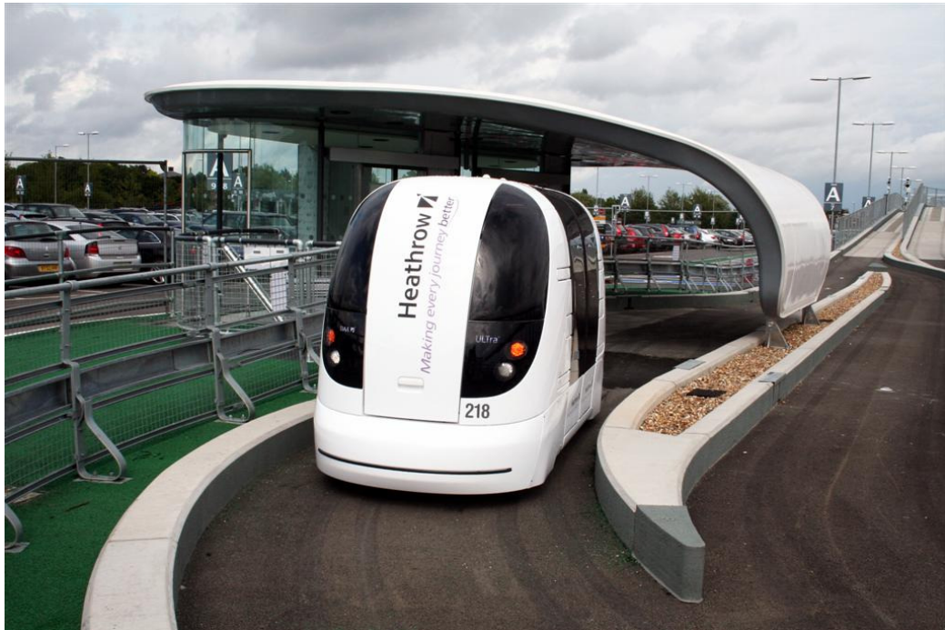
Figure 1.1: Photograph of a PRT vehicle and at-grade station at London Heathrow Airport. PRT vehicles, stations and infrastructure are smaller than typical Automated People Mover and urban rail systems. Vehicle length, width and height are 3.7m, 1.4m and 1.8m, respectively. Photo courtesy of ULTra PRT Ltd.
